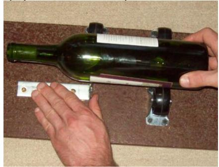
5. Place the larger corner brace behind the bottle in a center position until the cutter brace lines up to where you'd typically like to cut the bottle. For smaller bottles, you can re-screw this brace closer or place a wood block in-between as a spacer. (An even better solution will be to mount a bolt and threads on the brace so it can be adjustable.)
