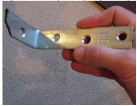
4. Now move that corner brace on the board with the bottle in the rollers until it fits correctly in place. Then screw that brace in place also.
