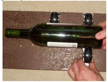
3. Take the smaller corner brace and place it around where the fourth wheel would go. Measure an estimated height for the brace and cut off with a angle grinder, cut off wheel, or reciprocating saw. Mine is cut at 2.5" inches from the bottom. When that is cut to height, half way through the top edge of the brace, cut about a 45 degree angle notch out. This will prevent the square edge from hitting the bottle.
