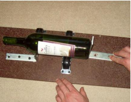
6. For this last step, you need to just position the cutter next to the cut brace and secure it with vice grips. If you have an oil feed glass cutter, make sure you don't use the vice grips on the cutter's head too hard. I accidently cracked mine!
