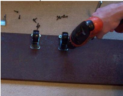
2. Place the third caster wheel on the opposite side of secured wheels and place various bottles that you will be cutting an in-between them. Move the castor wheel until the spacing allows for all typical bottle sizes that you are using such as a beer & wine bottle. The spacing for mine is about 2" inches from wheel edge to edge. Once in place, mount that wheel to the board with screws also.
