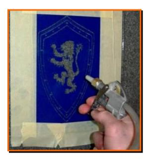
4. After it's etched evenly, peel off the stencil and masking tape.
