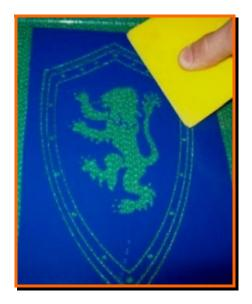
3. Third, take any type of sandblaster to surface etch the glass over the cut out areas of the stencil. Be sure to use abrasives that are as hard as the glass such as sand, aluminum oxide, or silicon carbide. I used about 30 pounds per square inch for the air pressure (30 PSI).
