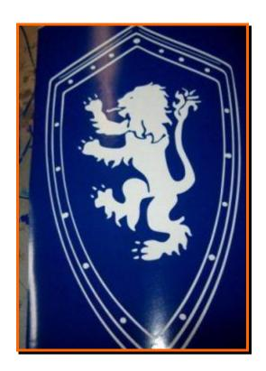
2. Second, I removed the backing paper from the stencil and aligned it on the flat piece of glass. You can see that I then used a squeegee to smoothly place the vinyl stencil while preventing any air pockets from developing. Make sure it's masked off around the edges to prevent over blast.
